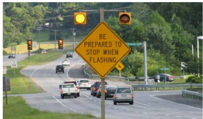
Example of Dynamic Signal Warning Flashers
